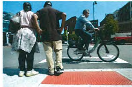
Figure 22. Pedestrian Detectable Warning Strips
