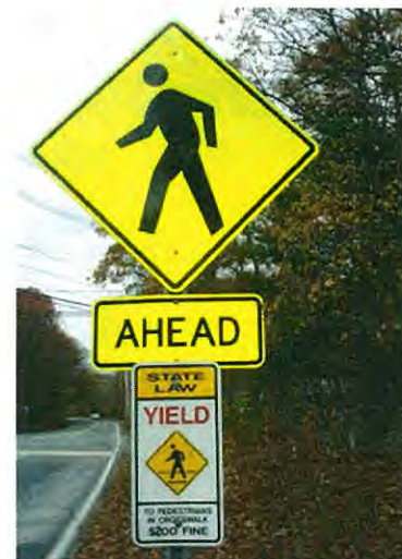
Figure 16. Pedestrian Advance Warning Sign
