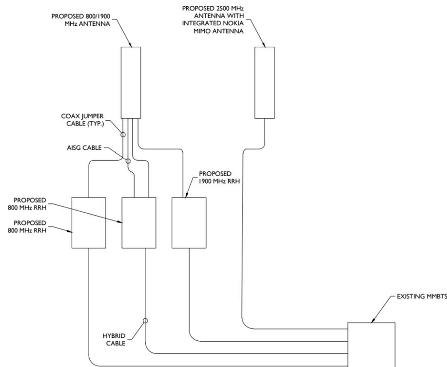
**ANTENNA WIRING DIAGRAM**
