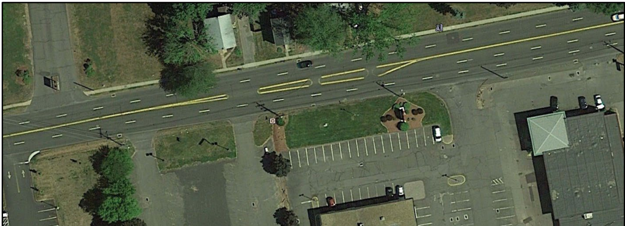
Excessive Curb Cuts (735-785 Silver Lane)
