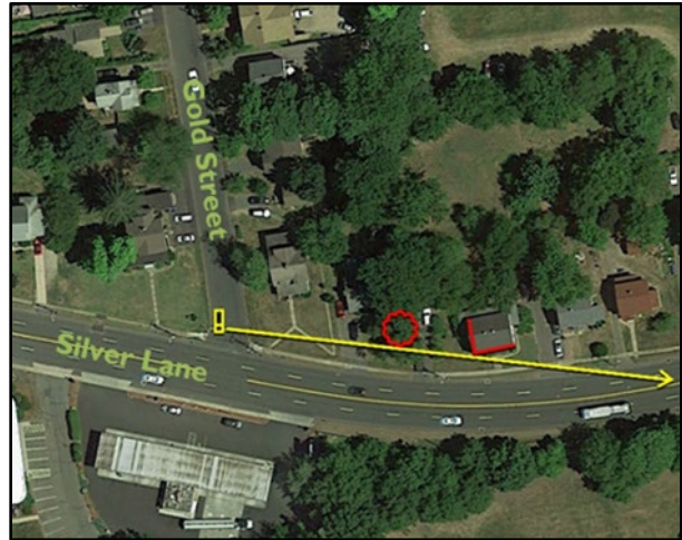
Limited Intersection Sight Distance at Gold Street
